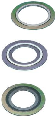
Spiral Wound gaskets are constructed by combining alternate windings of a pre-formed stainless steel with a filler material. Part of the manufacturing process involves spot welding the windings. These are known as an "R" type.
