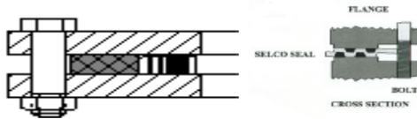
Note that most of the clamping force on a Spiral Wound (SW) is on the metal plate, not on the sealing element. They are self energized by system pressure, the pressure causing the "V" convolutions to open and therefore seal.
