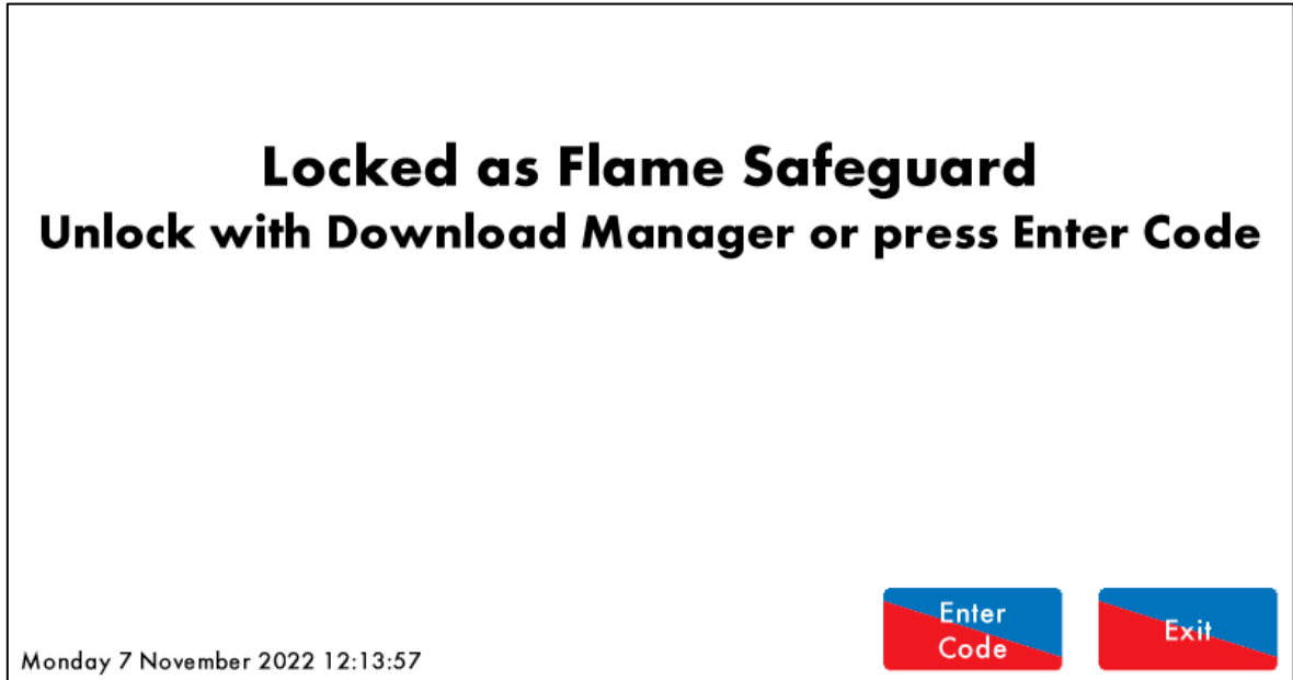
Figure 8.1.ii After pressing the Unlock button, you can upload the unlock code via Download Manager or Enter code.
